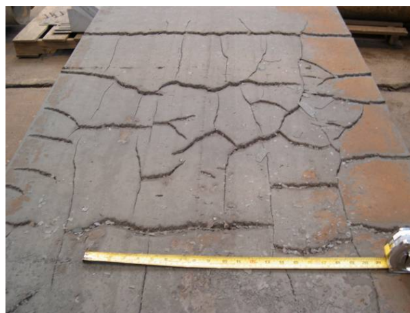
Fig. 1. Appearance of broken SK85 slab during hot rolling process.
